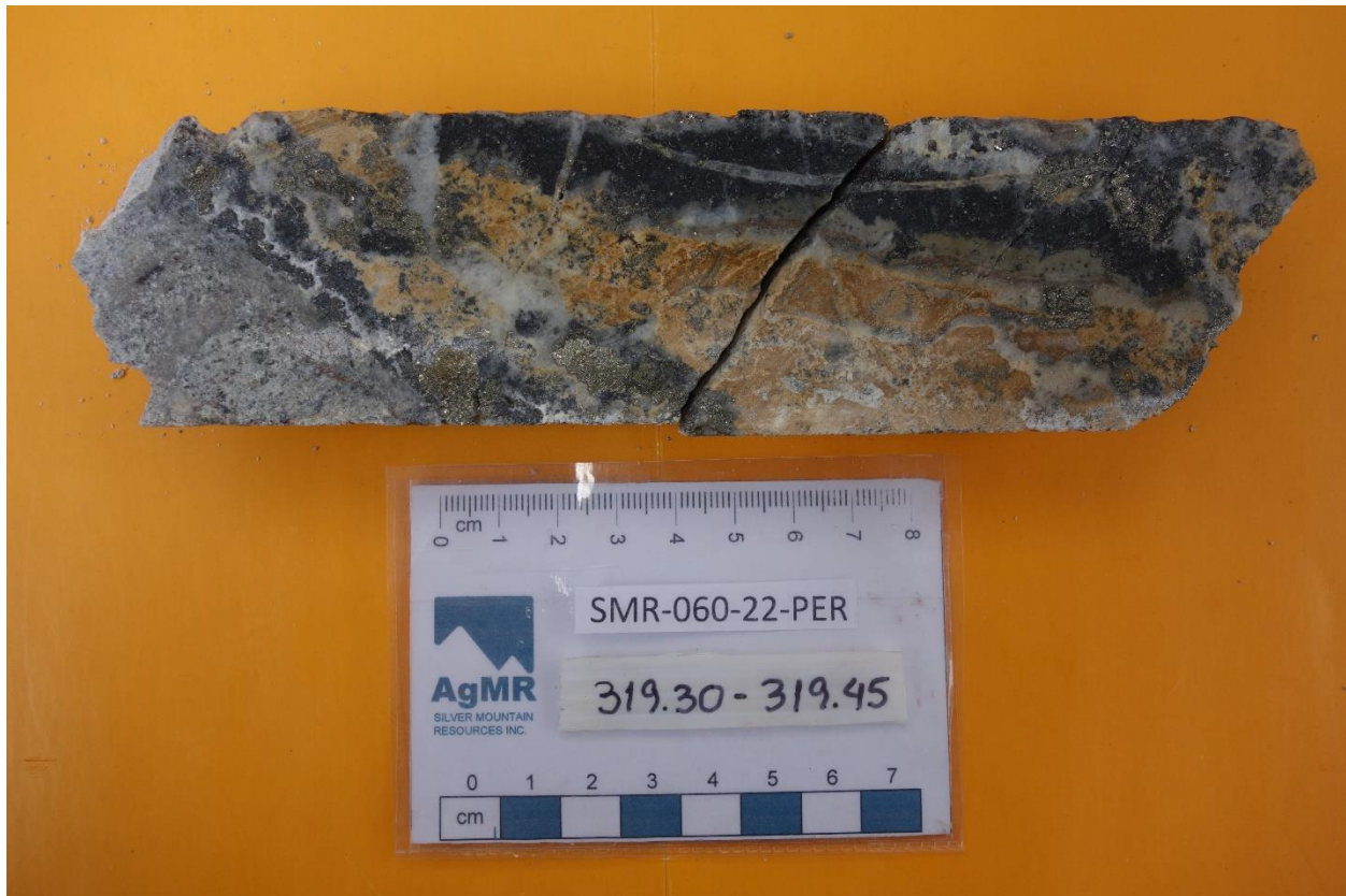
Fig.2: Photo of mineralized interval of drill core, Perseguida vein, hole SMR-060-22-PER, 319.30 – 319.45 m depth. Vein interval is composed of several generations of grey and milky white quartz, with irregular pods and fine veinlets of silver sulpho-salts, galena, sphalerite, chalcopyrite and pyrite. Late rhodochrosite with interspersed brown iron oxides is also visible.
